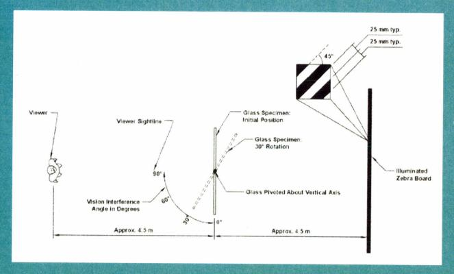
As described in the standard, inspection of glass is performed visually under strict guidelines as illustrated in Figure 2 of ASTM C1036, shown above.
