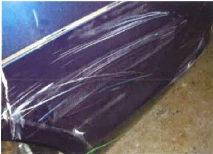
Figure 6: Photograph taken of the damages to the left (driver side) rear quarter panel.
