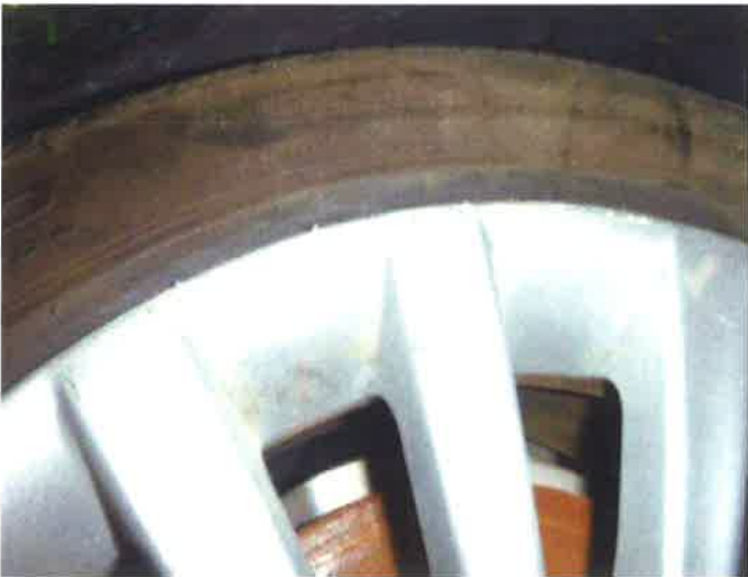
Figure 8: Close-up of the front left wheel cover. Note: There are no circumferential markings along the wheel cover to indicate the wheel was rotating at the time of impact.
