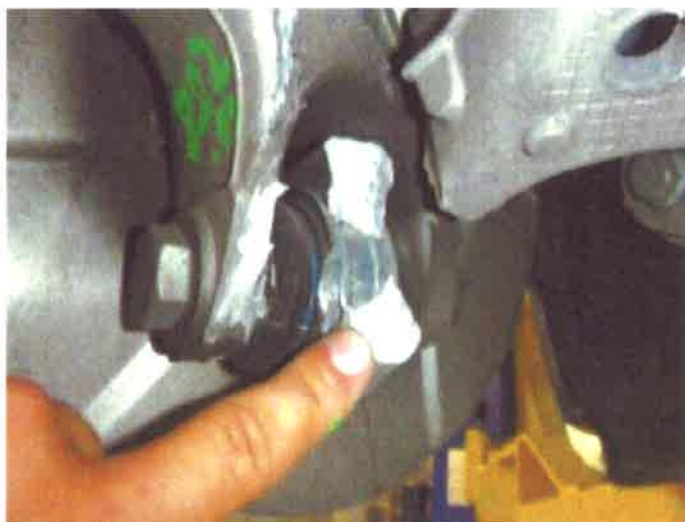
Figure 4: Close-up view of the reported damage to the lower left rear suspension control arm.
