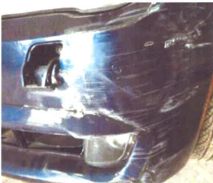
Figure 2: Reported damages to the front left (driver side) bumper cover on the BMW 750i sedan. Note: Scrape markings are all horizontal and straight, running parallel with each other.
