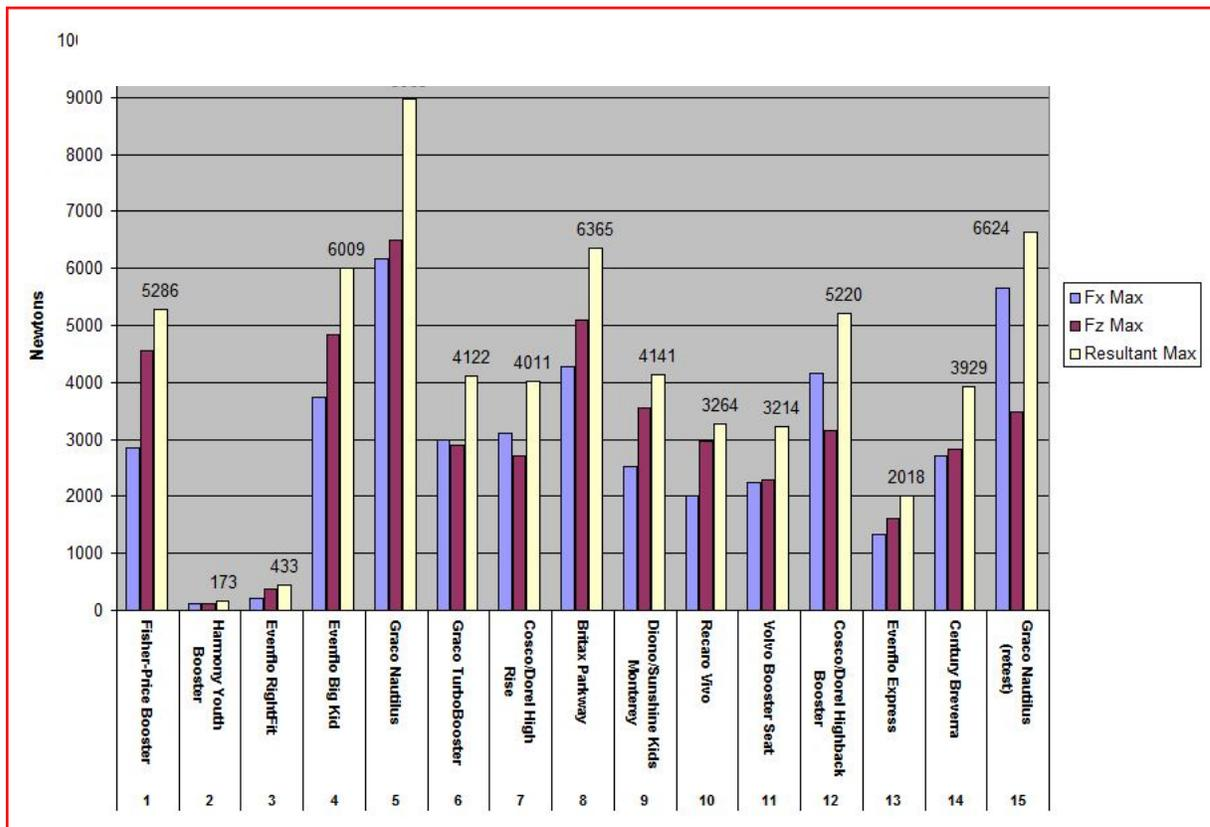
**Appendix E. Maximum Load Generated During Seat Bottom Pelvic Restraint Testing.**
