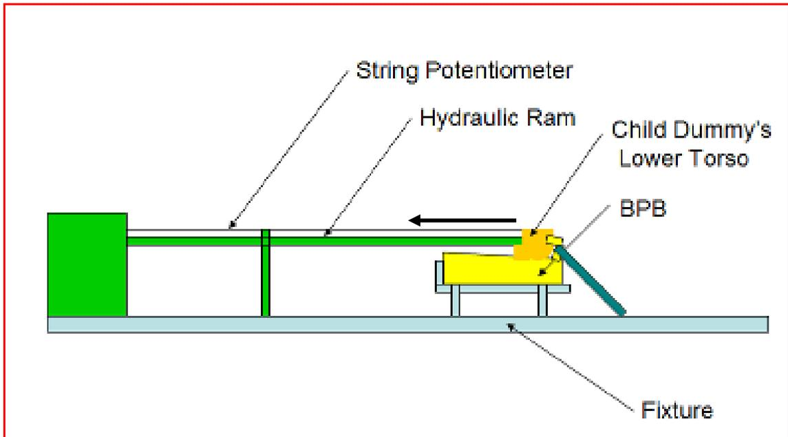
Appendix A. BPB Seat Surface Pelvic Restraint Test Set-up.
