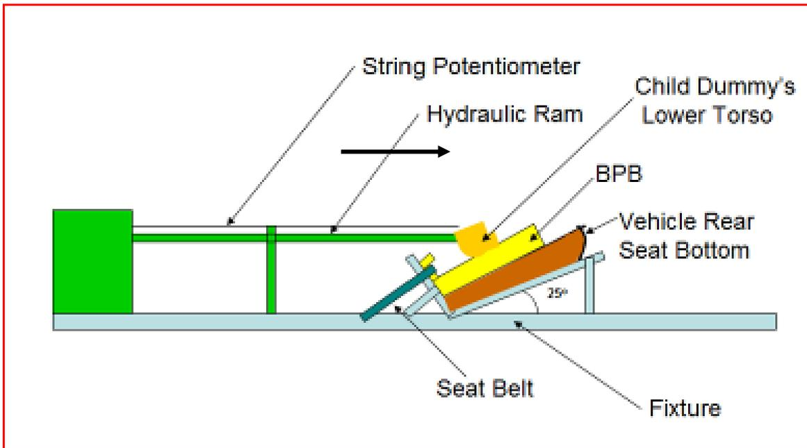
Appendix B. BPB Seat Bottom Compression Test Set-up.
