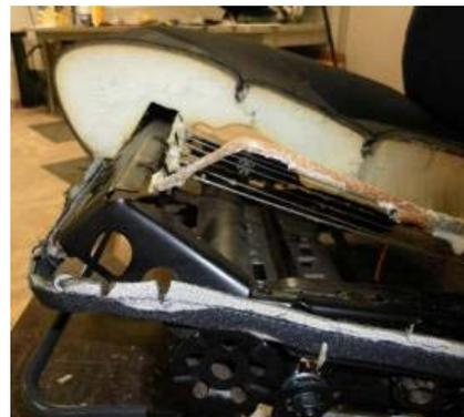
**Figure 1. 2001 Volvo S60 Right Front Seat Bottom Ramp.**
