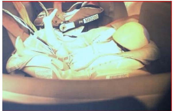
Figure 19. Ford Escape maximum forward excursion.
