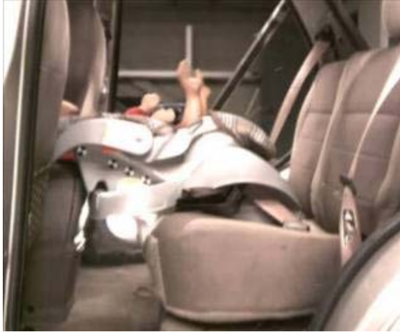
Figure 12. Test 2-1 Maximum Excursion.
