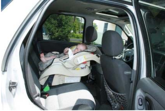
Figure 16. Exemplar CSS A Installed In Center Rear of an exemplar SUV.
