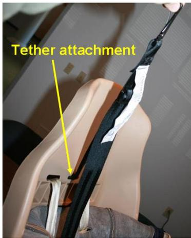
Figure 24. CSS A Low tether attachment
