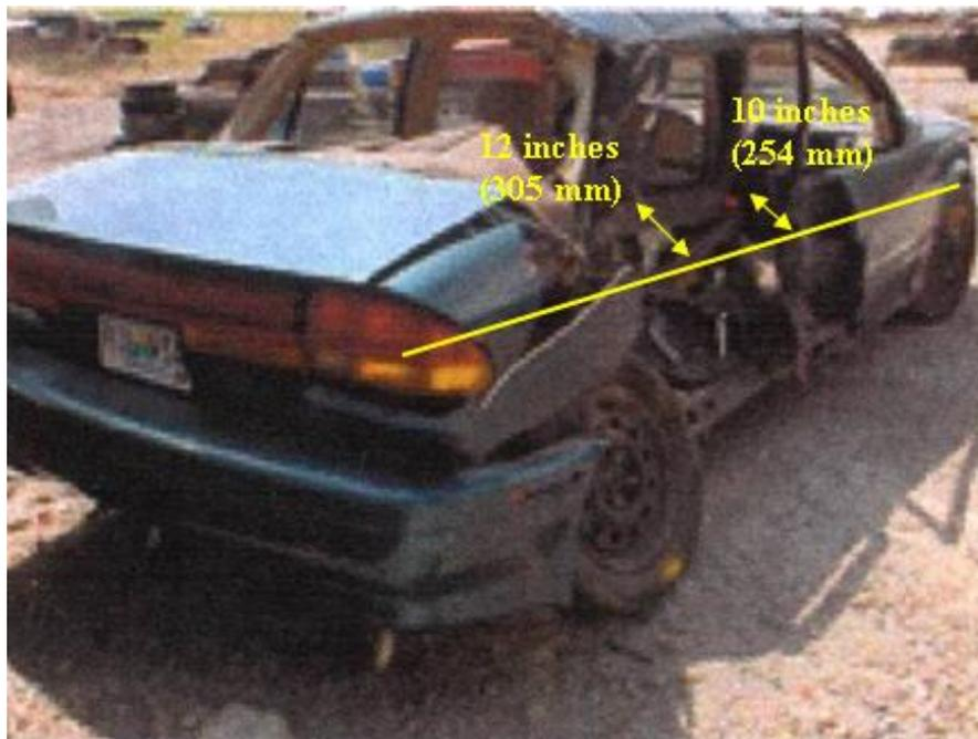
Figure 3. Intrusion to Saturn SL2 in Case 2
