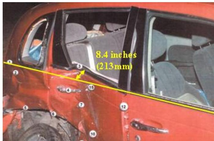
Figure 1. Intrusion into PT Cruiser in Case 1 crash
