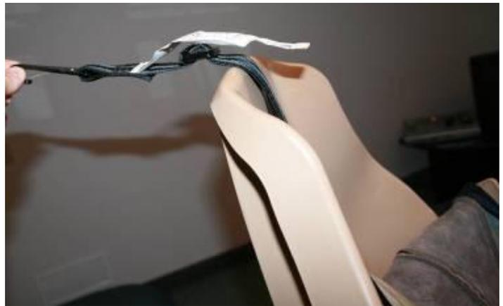
Figure 25. CSS A Tether routing over the top of the CSS seat back
