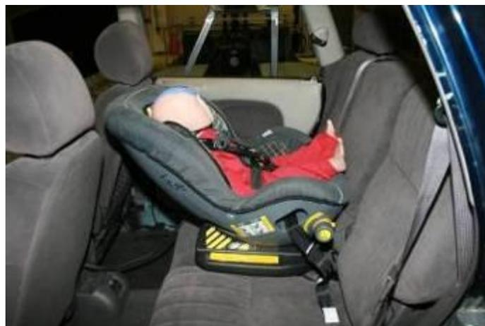
Figure 2. 12 month CRABI child dummy installed in an exemplar CSS installed in an exemplar PT Cruiser
