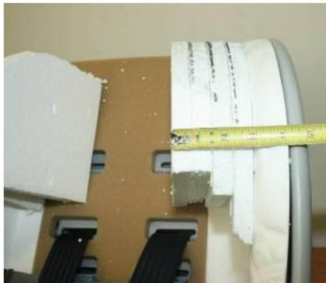
Figure 17. CSS C with 3 inches (76 mm) of EA padding added to the side wings
