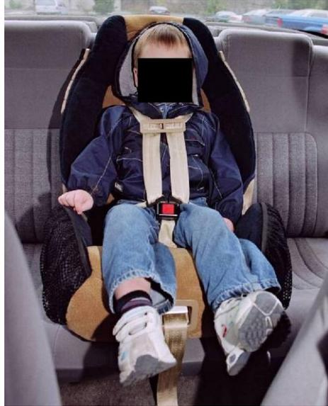
Figure 4. Surrogate child secured in an exemplar CSS in the rear center of an exemplar Saturn SL2
