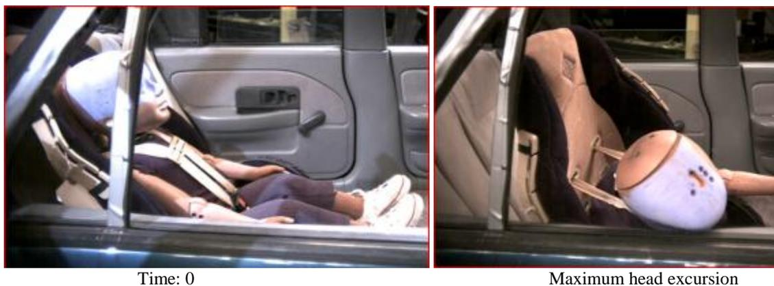
Figure 19. Maximum head excursion with untethered CSS A during Test 2.1
