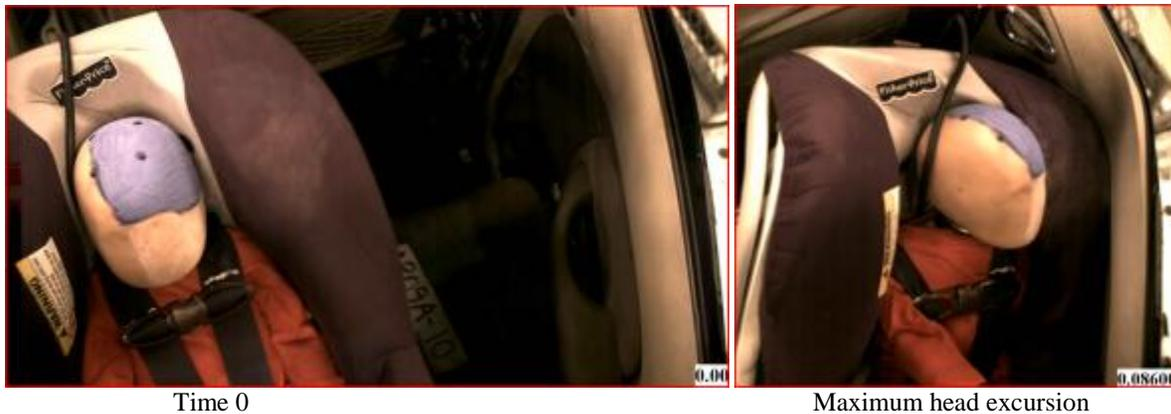
Figure 18. Maximum head excursion with CSS C incorporating modified side wings during Test 1.10
