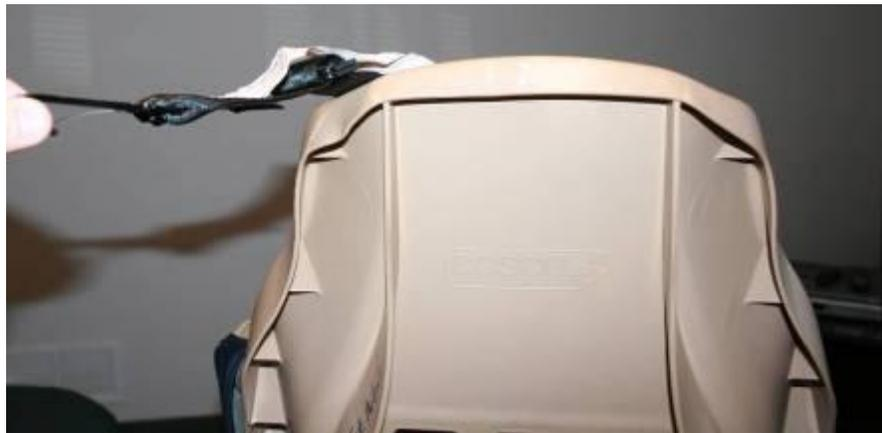
Figure 26. CSS A Tether slid laterally across the top of CSS1
