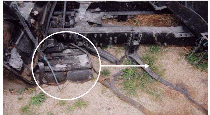
Photo 13 – Battery Box Moved Rearward
