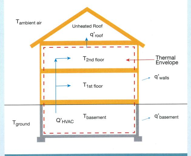
FIGURE 1: Example of Thermal Envelope, Temperatures, and Heat Transfer
