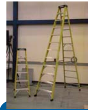
Photo 1: This experiment used 6-ft and 12-ft Type 1A fiberglass ladders.
