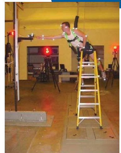
Photo 2: A participant reaches toward the target from a 6-ft stepladder.
