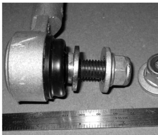
Figure A: Newly purchased replacement end link with included hardware that includes the proper captive nut with insert
