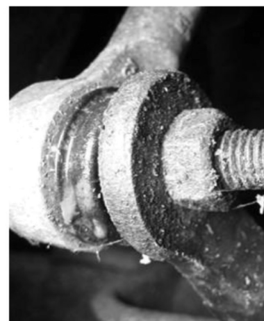
Figure B: Improper hardware used on left rear link
