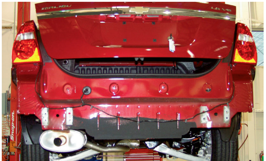
Figure 11 – Case Study 2, Trunk area of the IIHS tested Chevrolet Malibu at 5 mph, showing no deformations to the trunk area
