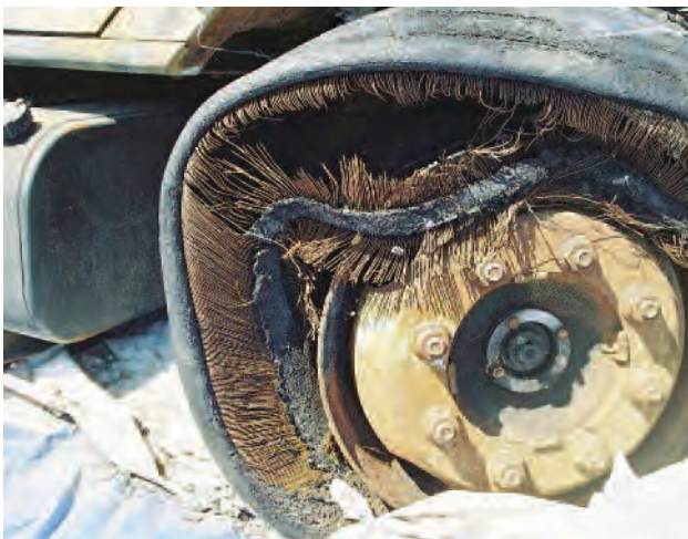
Photo 24: Straight tire cords indicating no rotation at time of fire.
