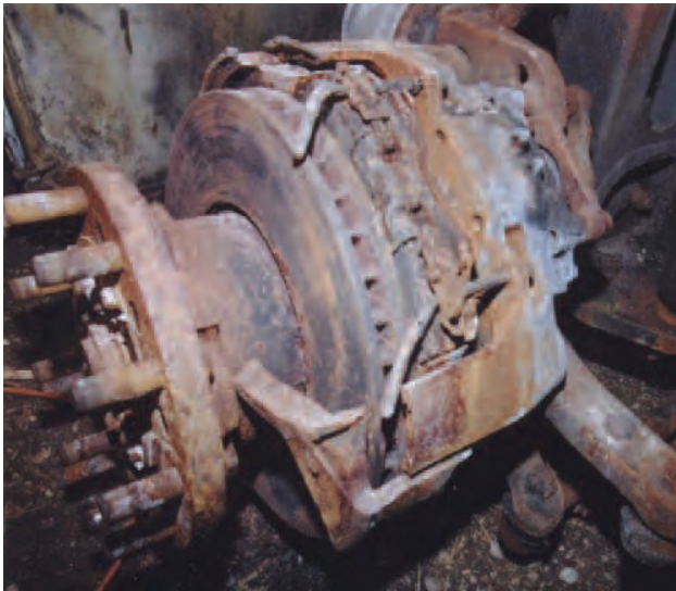
Photo 16: Causal disc brake/wheel end failure.
