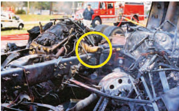
Photo 5: (right) Turbocharger with impact damage.
