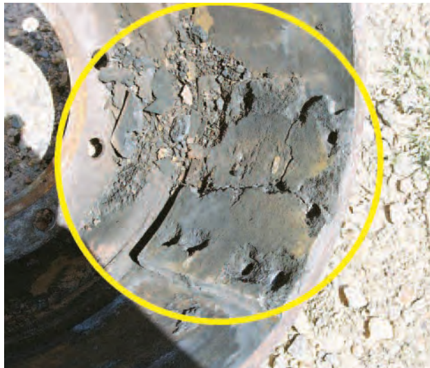
Photo 22: Fused brake block
