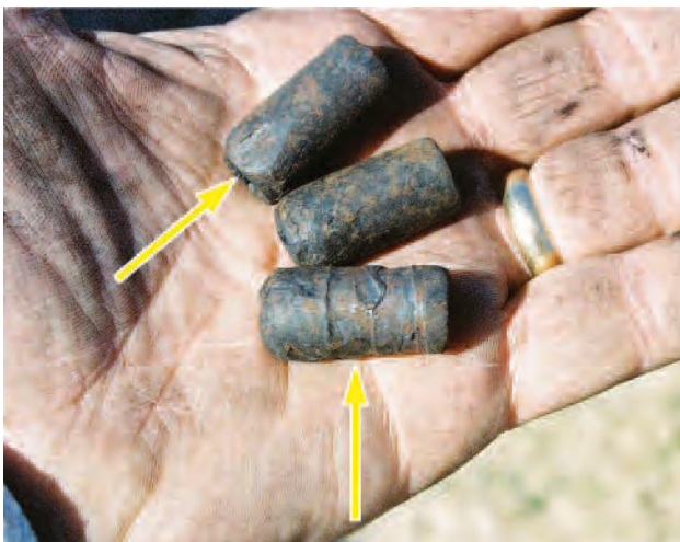
Photo 14: Deformed bearing rollers.
