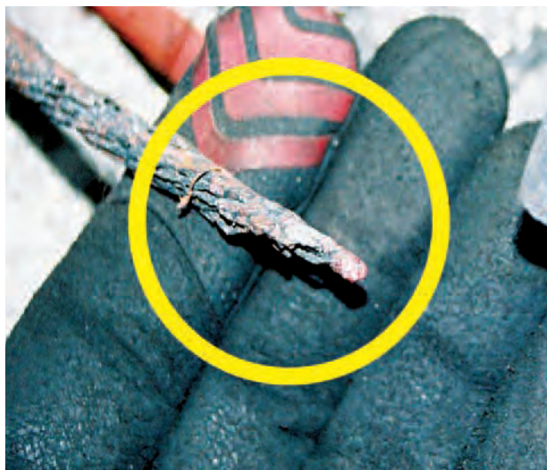
Photo 29: Example of "balling" phenomenon.
