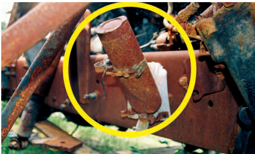
Photo 33: Starting fluid canister shows impact damage.
