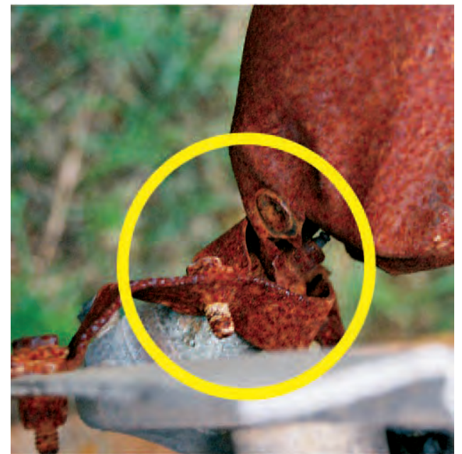
Photo 34: Starting fluid canister (breached).
