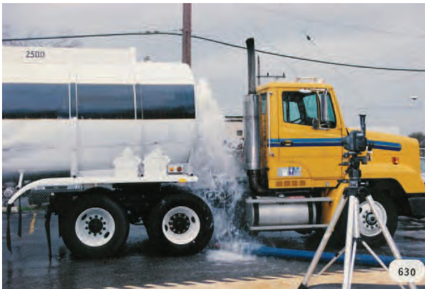
Photo 32: Full-scale testing of fuel breach.
