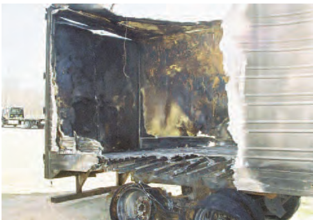
Photo 13: Hub failure/tire fire.
