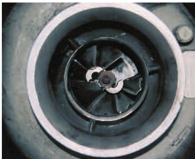
Photo 25: Failed turbocharger compressor.
