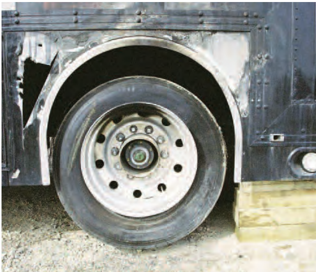
Photo 19: Tire fire started by dragging parking brake.
