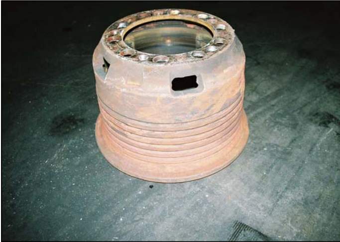
Photo 12A: Brake Drum Rouging Caused by Overheating
