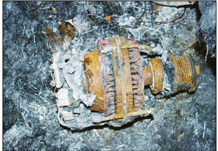
Photo 4A: Causal Alternator
