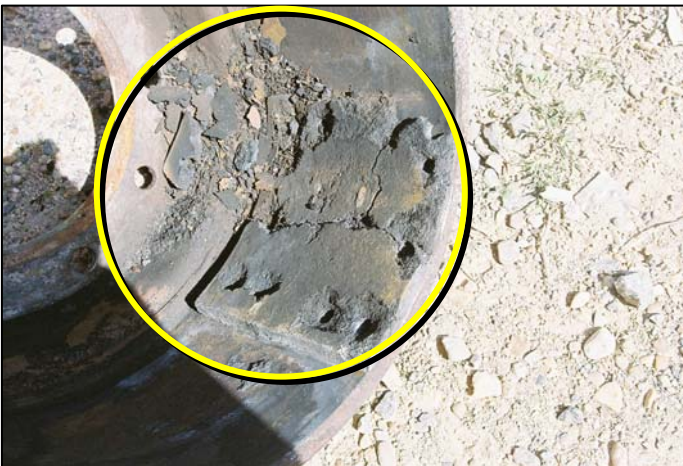
Photo 13: Fused Brake Block
