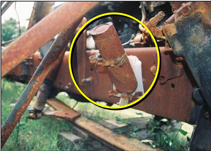
Photo 24A: Starting Fluid Canister-Impact Damage
