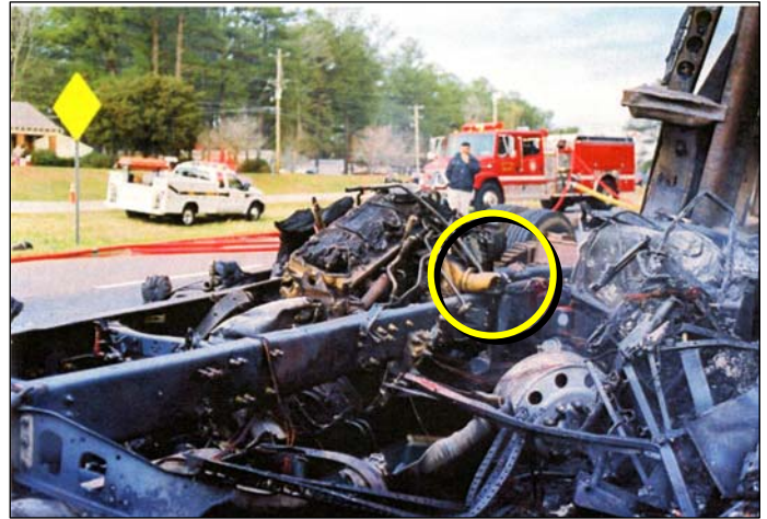
Photo 3A: Turbocharger, Impact Damage
