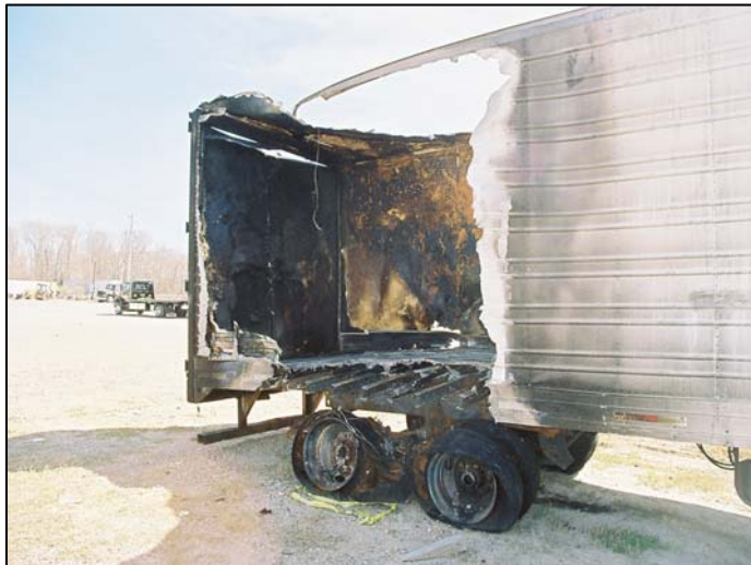
Photo 6: Hub Failure/Tire Fire
