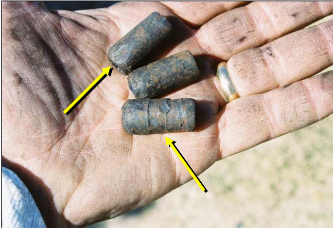
Photo 7A: Deformed Bearing Rollers
