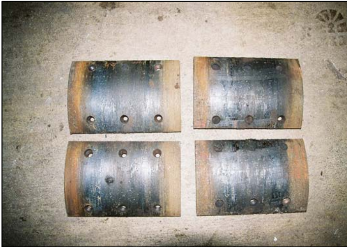
Photo 12B: Drum Brake; Brake Blocks Overheated
