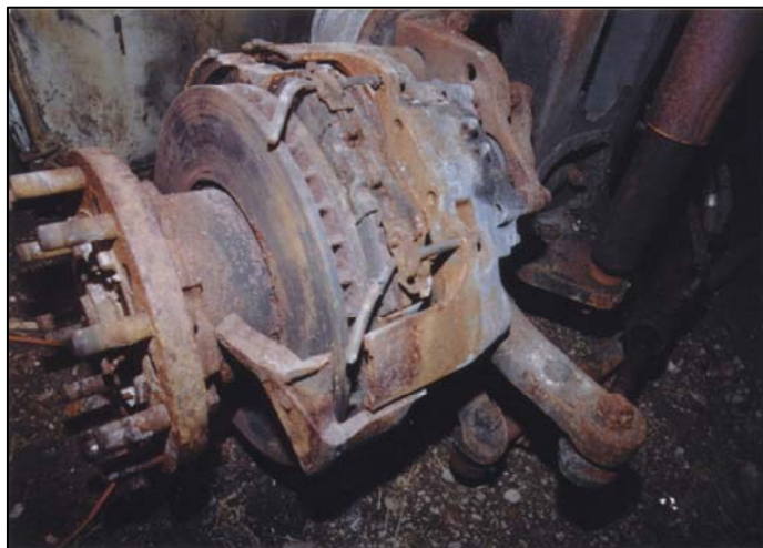
Photo 8: Causal Disc Brake/Wheel End Failure
