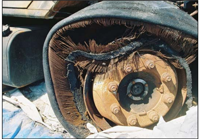
Photo 15: Straight Tire Cords Indicating No Rotation at Time of Fire
