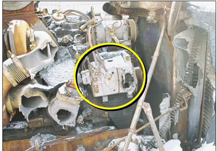
Photo 4B: Non-Causal Alternator
