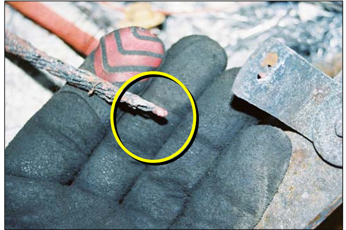
Photo 20: Example of "Balling" Phenomenon
