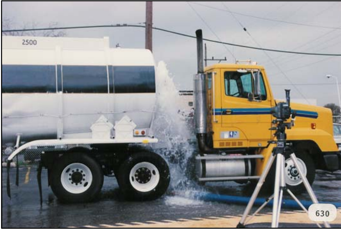
Photo 23: Full Scale Testing of Fuel Breach
