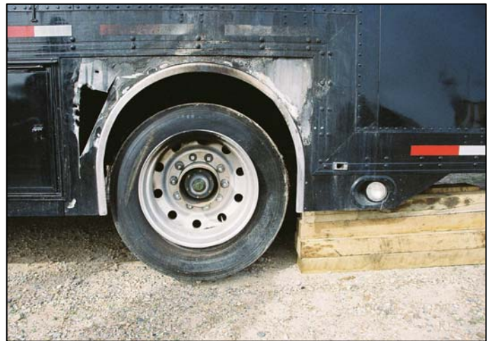
Photo 11: Tire Fire Started by Dragging Parking Brake
